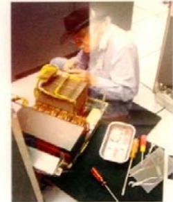
Restoration team member Bob Erickson works on the challenging task of repairing the machine's core memory unit. Bob was an IBM customer engineer from 1941 to 1984.
