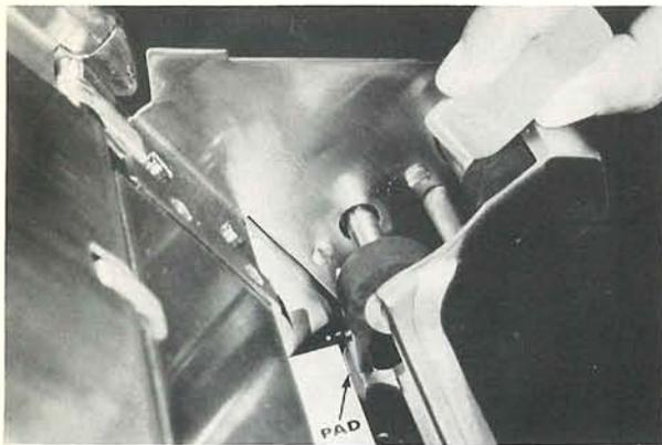
GLAZED RUBBER ROLLERS in the file feed may cause misalignment of the cards in the hopper and subsequent card jams. Roughen any glazed rollers with a typewriter eraser. Check also that the FILE FEED CLUTCH is tripped as soon as the level of the card deck falls below the front jogger pad.
