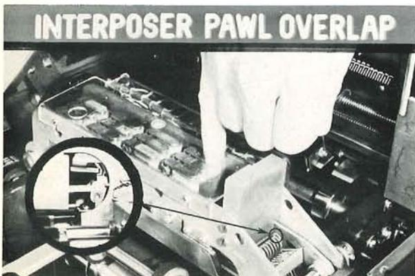
THE SELECTOR UNIT timing. Always check this item first. Ensure that there is sufficient overlap between the interposer pawl and the selector bail so that the pawl cannot slip off. Check this at both ends of the selector unit for the 9 and 12 interposers. Here is an opportunity to check dynamically with the STROBOSCOPE.
