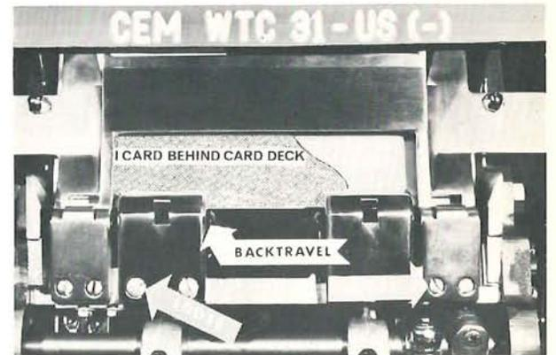
**083 FEED KNIVES** do not usually wear. Excessive end play of the knife blocks on their pivot studs can be cured by shimming. Feed knife blocks which bind on the pivot stud, due to too small diameter of the hole, must be replaced. Sharp rear edges on plastic knives may tear zero-holes in the path of the knives. Stone these edges to overcome this problem.
