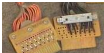
Figure 17: Edge Connectors (aka Paddle Cards)
