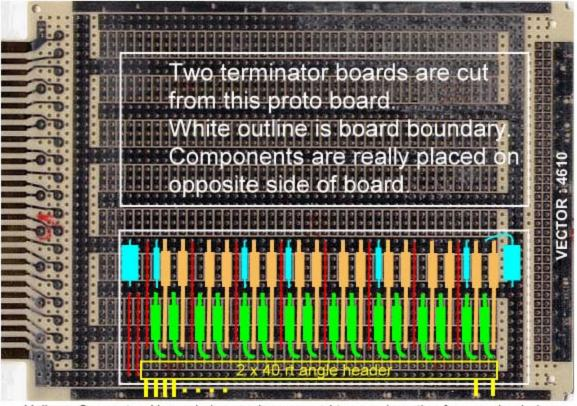
Yellow - Connector. Unused pins can be removed to ease insertion force and polarize the connector. About 1/3rd of pins are unused.
